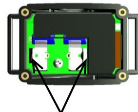
Reset: connect the 2 battery supports
