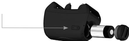
Diagram 4 Fitting the battery in the receiver collar
