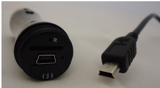
Diagram 1 USB port to charge the battery
