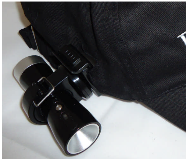
Diagram 6 Fitting the video cam to the EYENIMAL® cap
