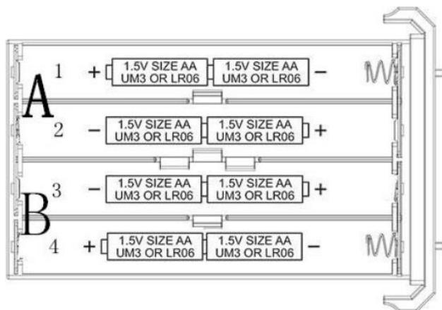
The working voltage of the camera is 12V. To supply power for the camera, 8 AA (LR06) batteries are needed.
