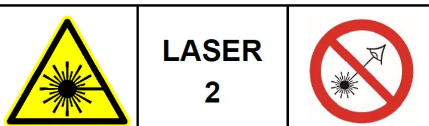
LASER RADIATION DO NOT STARE INTO BEAM
