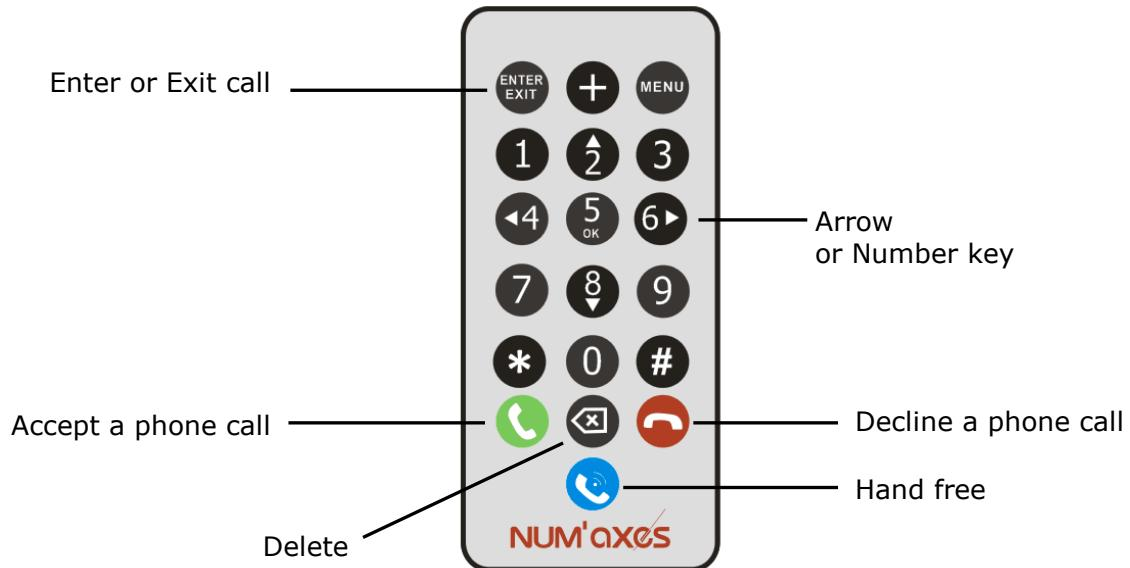
The remote control is used for customer settings and phone function. It is an infrared type wireless remote control and its range is a few meters. Point the remote control towards the front of the camera.
