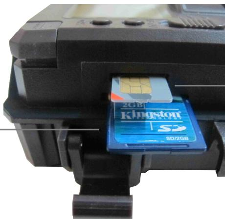
Insert the SD card with the label facing upward and the contacts facing downward.
