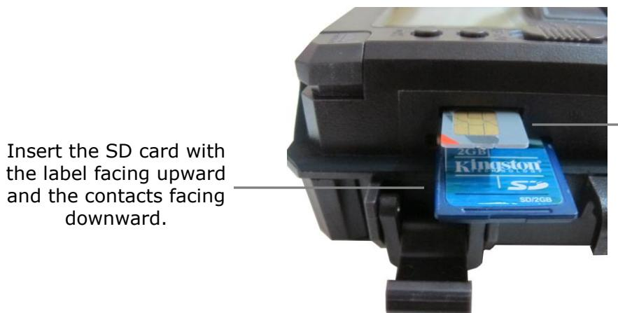
Insert the SD card with the label facing upward and the contacts facing downward.
