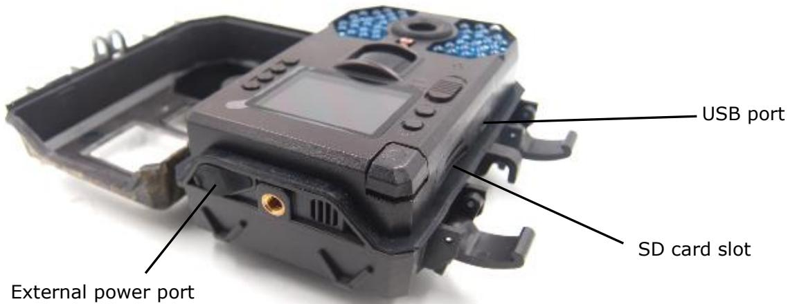
The camera provides the following connections for external devices: USB port, SD card slot and external power connector.
