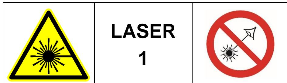
LASER RADIATION DO NOT STARE INTO BEAM
